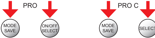
figure 13 Push down both buttons of the lubricator at the same time > 4 s.
